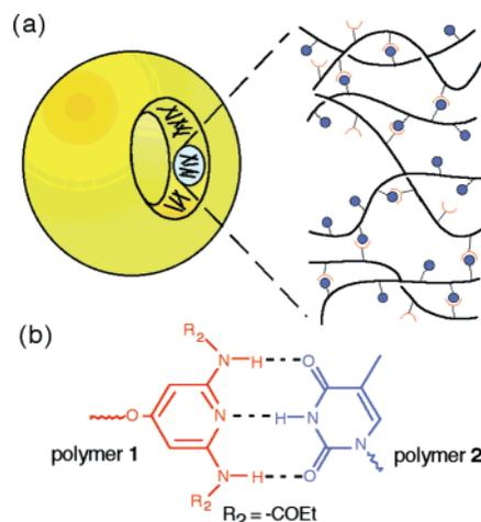
**Figure 2.** Schematic demonstration of vesicle formation between diaminopyridine-based polymer **1** and thymine-based polymer **2**. (a) Illustration showing molecular recognition within vesicle wall. (b) The corresponding recognition dyads.
