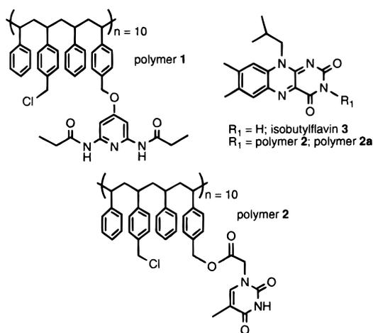
**Figure 1.** Schematic showing diaminopyridine-based polymer **1**, thymine-based polymer **2**, and partially functionalized polymer **2a** (10% by functional group number). Polymers were prepared from poly-*co*-[4-(chloromethyl)styrene-styrene];  $M_n = 5300 \text{ g mol}^{-1}$ .
