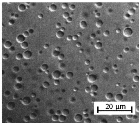
**Figure 3.** DIC micrograph ( $\times 60$ ) clearly showing the spherical aggregates that were obtained in  $\text{CHCl}_3$ . Solutions were prepared from 1 equiv of **1** and 1 equiv of **2**.  $[\mathbf{1}] = [\mathbf{2}] = 3 \text{ mg/mL}$ .
