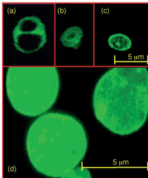
**Figure 5.** Confocal micrographs of varying architectures in  $\text{CHCl}_3$ , showing the vesicle nature of these mixed-polymer systems. (a) ( $\times 60$ ) Fused-vesicle morphology; (b) ( $\times 60$ ) vesicle-in-vesicle structure; (c) ( $\times 60$ ) regular spherical vesicle morphology; (d) ( $\times 120$ ) two spherical vesicles and a fused vesicle. Prepared from 6 equiv of **1**:5 equiv of **2**:1 equiv of **2a**.  $[\mathbf{1}] = [\mathbf{2}] = [\mathbf{2a}] = 3 \text{ mg/mL}$ .
